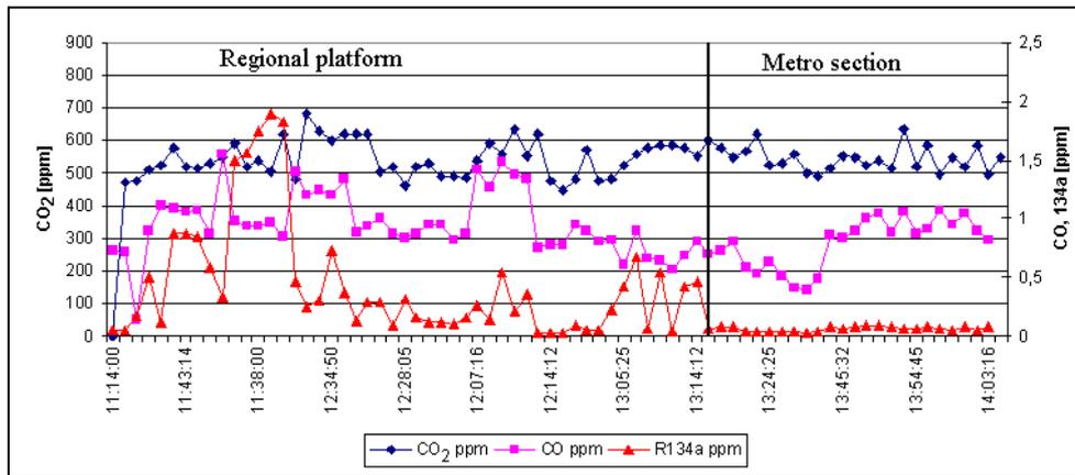
Fig.5 The results measured by the ventilation monitoring system as displayed by the Application Software 7620
