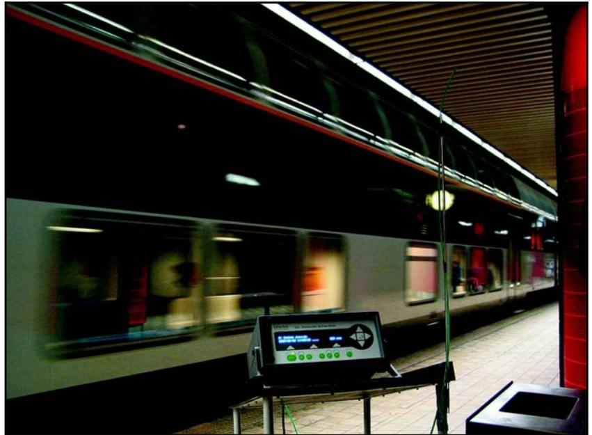
Fig.1 Monitoring CO, CO<sub>2</sub> and Freon 134a in a subway station in Copenhagen
