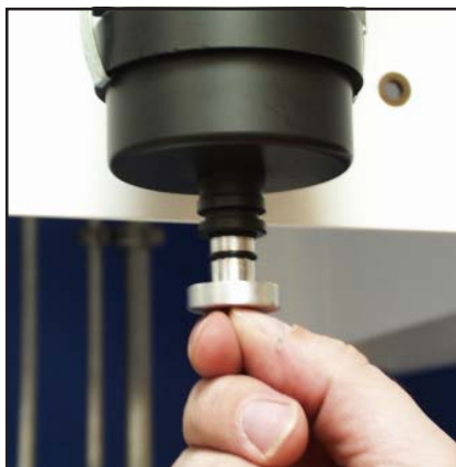
Insertion of Leak Check Plug.
