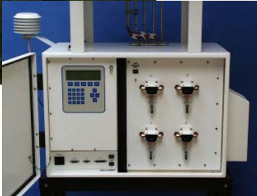
The Speciation Sampler Shares the Same User Interface with the Partisol-Plus Sequential Air Sampler.
