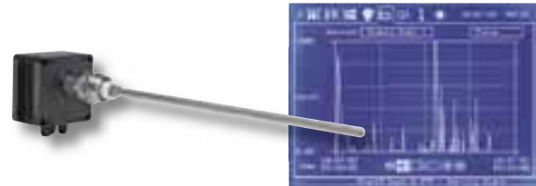
Dynamics of dust levels during bag cleaning shown with graphics screen
