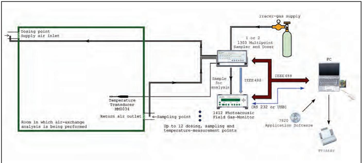
Fig.2 A typical air-exchange analysis system, shown with an application example. In this case, the aim of the analysis is to determine the size of the air-change in the mechanically ventilated room. The diagram shows only one dosing and sampling point, for clarity. Up to six similar analyses can be performed simultaneously using one 1303. Application Software 7620 gives control of all the functions of the system.
