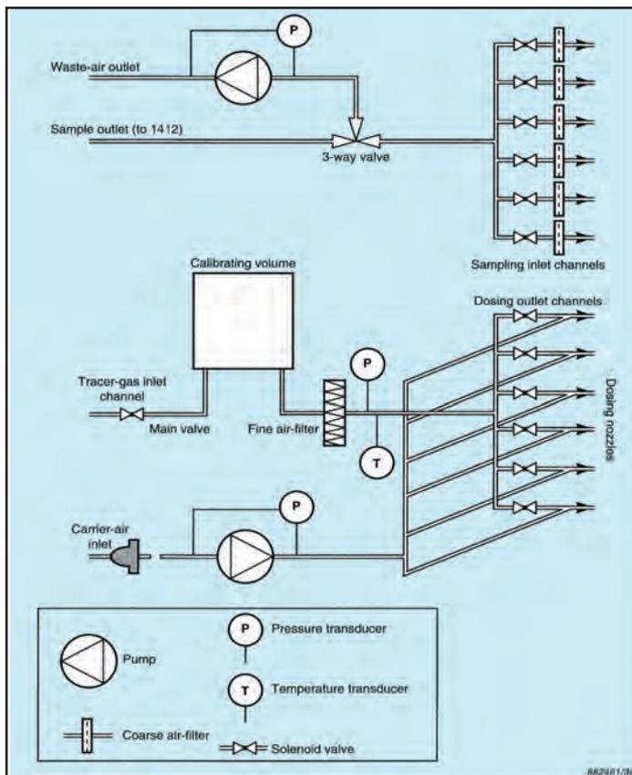
Fig.1 A schematic diagram of the 1303's pneumatic system: the sampler system is depicted at the top, the doser system at the bottom. The use of non-reactive materials throughout minimizes gas adsorption in the internal air-channels.
