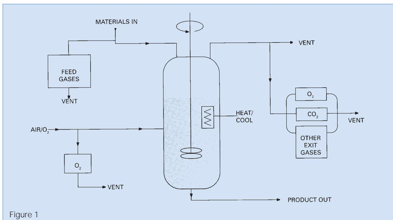
The measurement of oxygen and other gases is often required to ensure the efficient operation and control of fermenters. Servomex can supply paramagnetic and infrared analysers complete with sample conditioning systems to continuously monitor these gases with little operator intervention.
