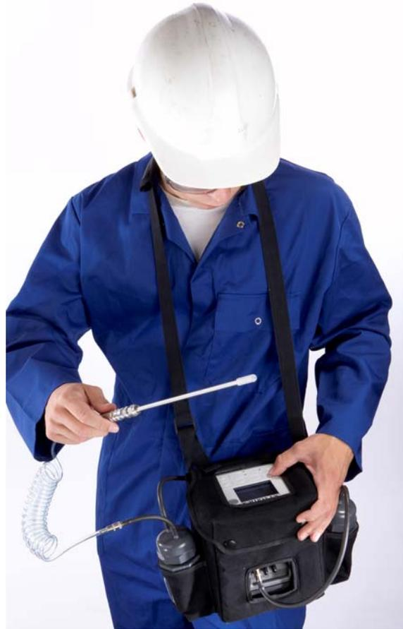
***Customers can now benefit from a wide range of accessories and options for the intrinsically safe Servomex 5100 i.s portable gas analyser. Extra options include an internal pump and a flexible sample tube, a sample gas conditioning kit approved for use in hazardous areas and a filter and probe holder assembly. The unit is also fitted with a carrying strap for ease of use and can also be supplied with an optional soft carry case.***
